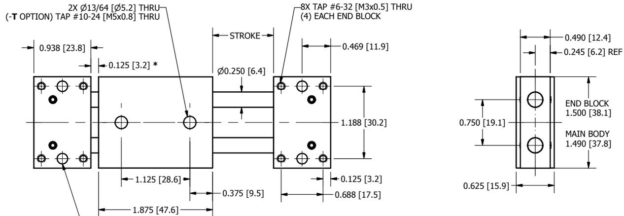
\* NOTE : 0.125 [3.2] HAS BEEN ADDED TO OVERALL STROKE TO PREVENT CONTACT BETWEEN MAIN BODY AND END BLOCKS WHILE OPERATING IN STANDARD STROKE RANGE
