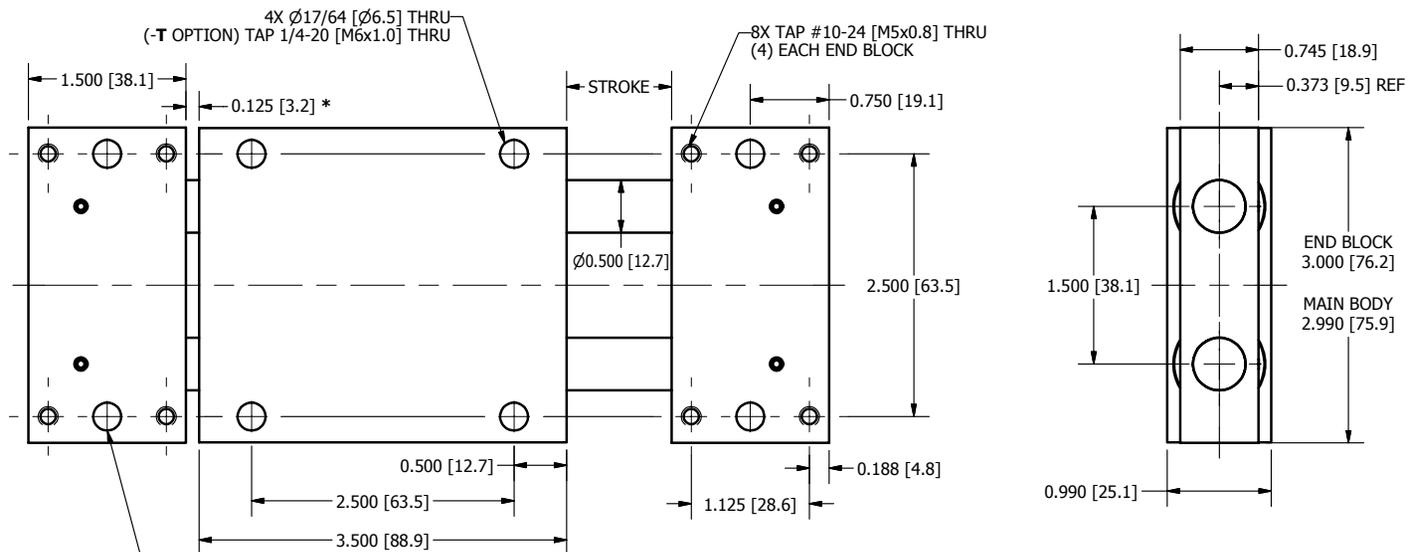
\* NOTE : 0.125 [3.2] HAS BEEN ADDED TO OVERALL STROKE TO PREVENT CONTACT BETWEEN MAIN BODY AND END BLOCKS WHILE OPERATING IN STANDARD STROKE RANGE
