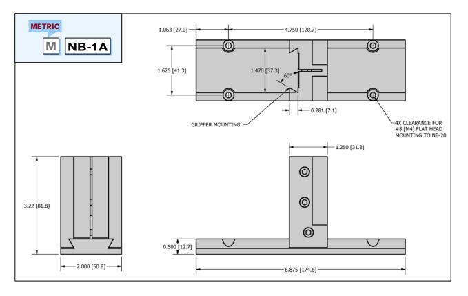
Use the **NB-1A** adjustable tooling to mount the following **DURA**-GRIP grippers to **NB-20**
